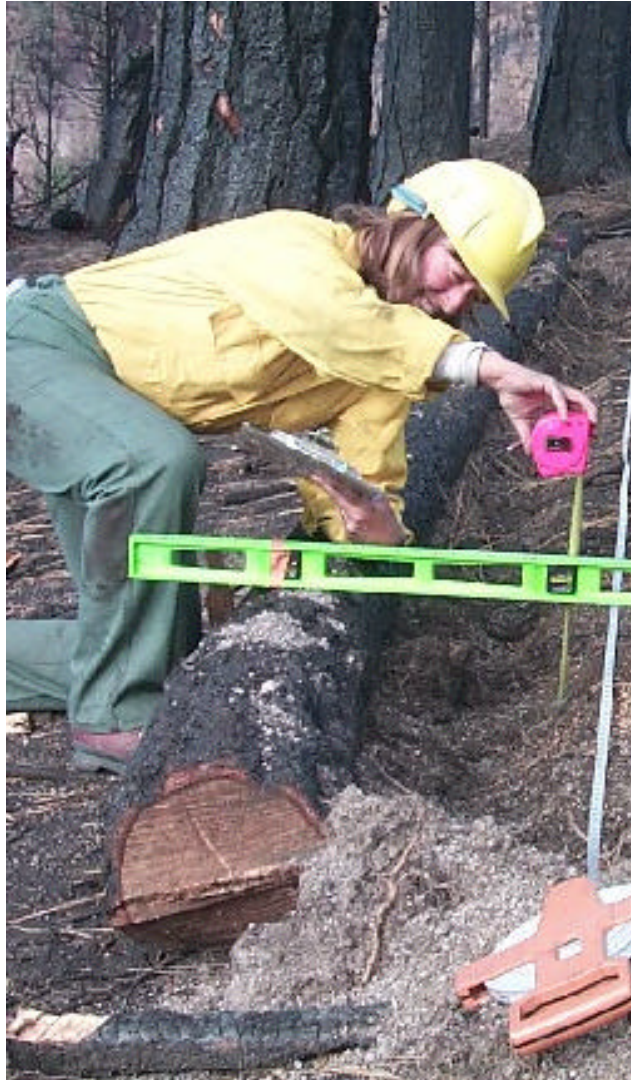
Figure 4. Measuring the sediment storage capacity behind a contour felled log. shows that the logs collect about half of the detached sediment from each storm, until their capacity is reached. The capacity can be estimated from the relationship:
