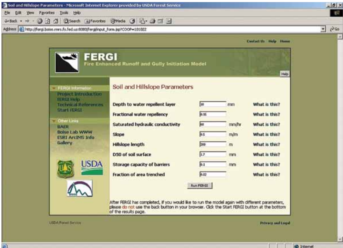
Figure 17—FERGI soil and hillslope input screen.
