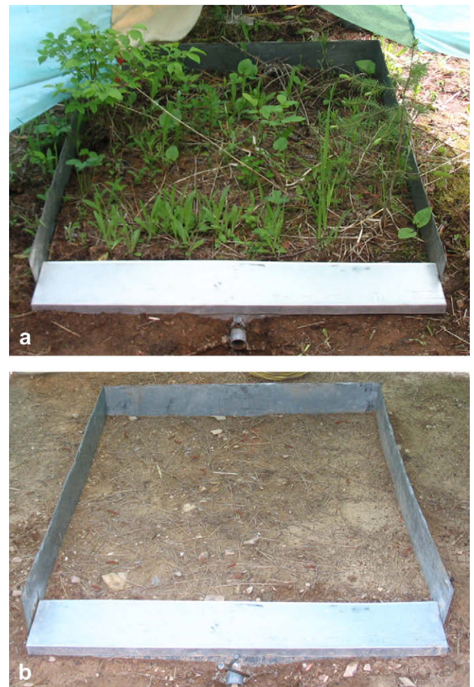
Fig. 2. Rainfall simulation plots (1 × 1 m) installed in the non-track portion of a brushed-in road (a) and the non-track portion of a reopened road (b) in northern Idaho, USA.
