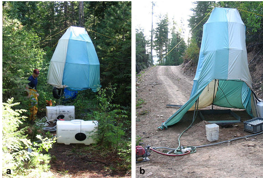
Fig. 1. Portable rainfall simulator assembled on a brushed-in road (a) and a reopened road (b) in northern Idaho, USA.
