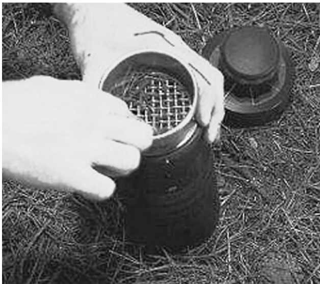
Fig. 2. The duff sample is pulled from the lower duff layer and pushed by hand through the sieve directly into the sample chamber. Rocks, sticks and larger needles stay in the sieve while smaller, more decomposed pieces of duff fall into the sampling chamber.
