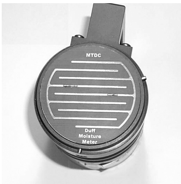
Fig. 4. The bottom of the sample chamber has two interlocking finger electrodes, spaced 6 mm (0.24 in) apart, etched onto a Teflon circuit card and attached to a movable plate made of low-dielectric plastic.
