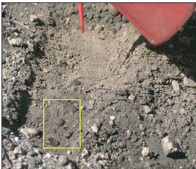
Figure 1 —The water drop penetration time (WDPT) test performed at 1 cm below the surface of the soil. The water drops inside the rectangle are beaded up on the surface while drops outside of the rectangle have infiltrated the soil.
