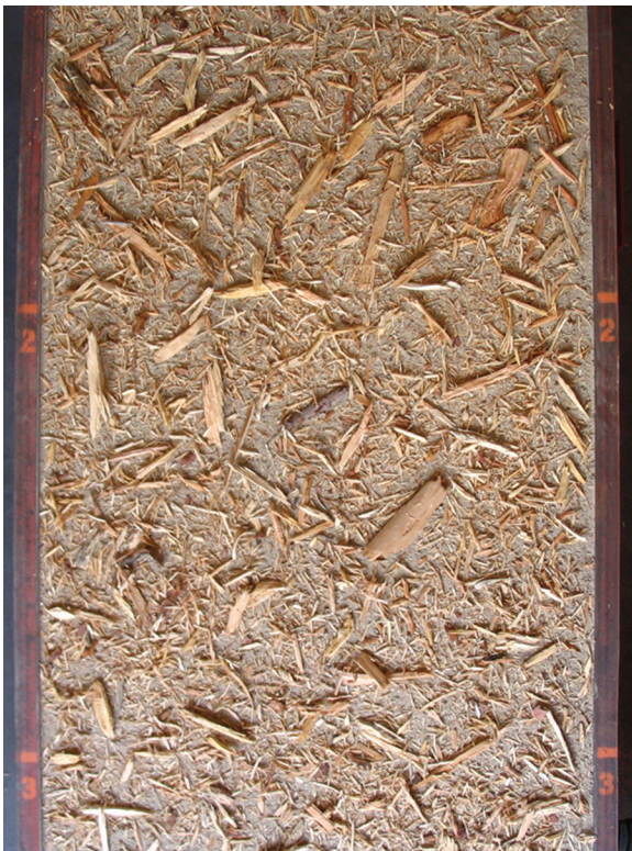
Figure 1. A portion of the rainfall and overland flow simulation laboratory plot with a 70 percent cover of wood shred mulch.
