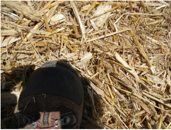
Figure A5. Wood shreds and agricultural straw mixed in staging area prior to loading into cargo net.
