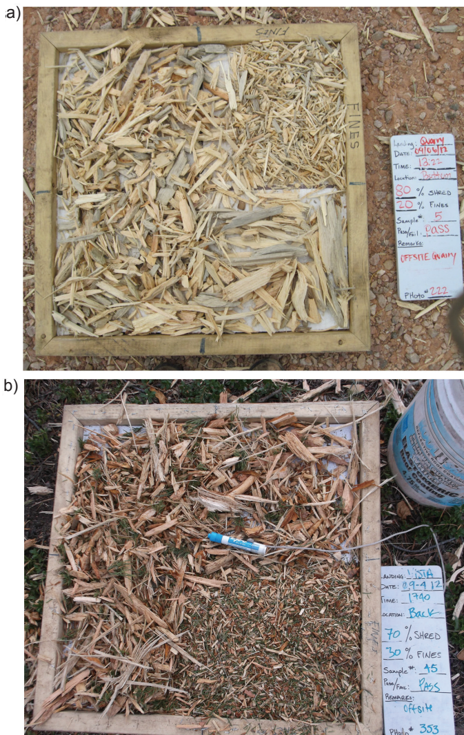
Figure B1. Two wood shred samples that passed inspection for BAER treatment implementation at the 2012 Waldo Canyon Fire. Both samples had been screened and are shown distributed in the quadrants of the sample frame. Note that sample b) contains green needles and is generally more finely shredded as compared to a).
