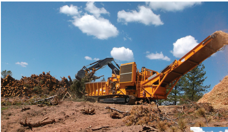
Figure 3. Wood being fed into a horizontal grinder to produce wood shreds at the 2012 Waldo Canyon Fire.
