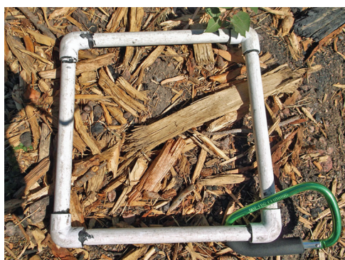
Figure 9. Ground cover assessment of aerially applied wood shred mulch at the 2012 Waldo Canyon Fire.
