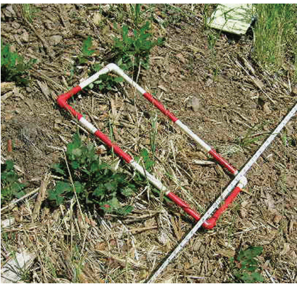
Figure 8. Ground cover of wood shred mulch being measured on a steep slope at the 2010 Schultz Fire.
