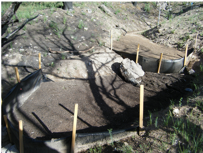
Fig. 3. Sediment captured by sediment retention structures in catchment I from a rain event on 8 July 2011 (12 mm total, I_{30} = 14 mm h^{-1} ).
