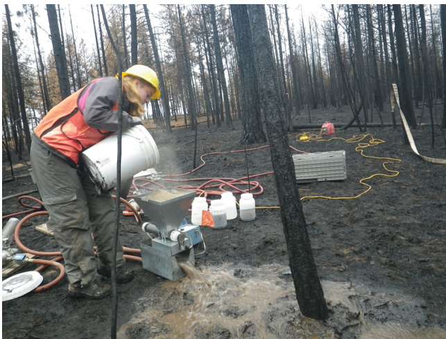
FIGURE 3 Sediment being added to the sediment hopper which was calibrated to add 25 g/L of sediment to the three flow rates
