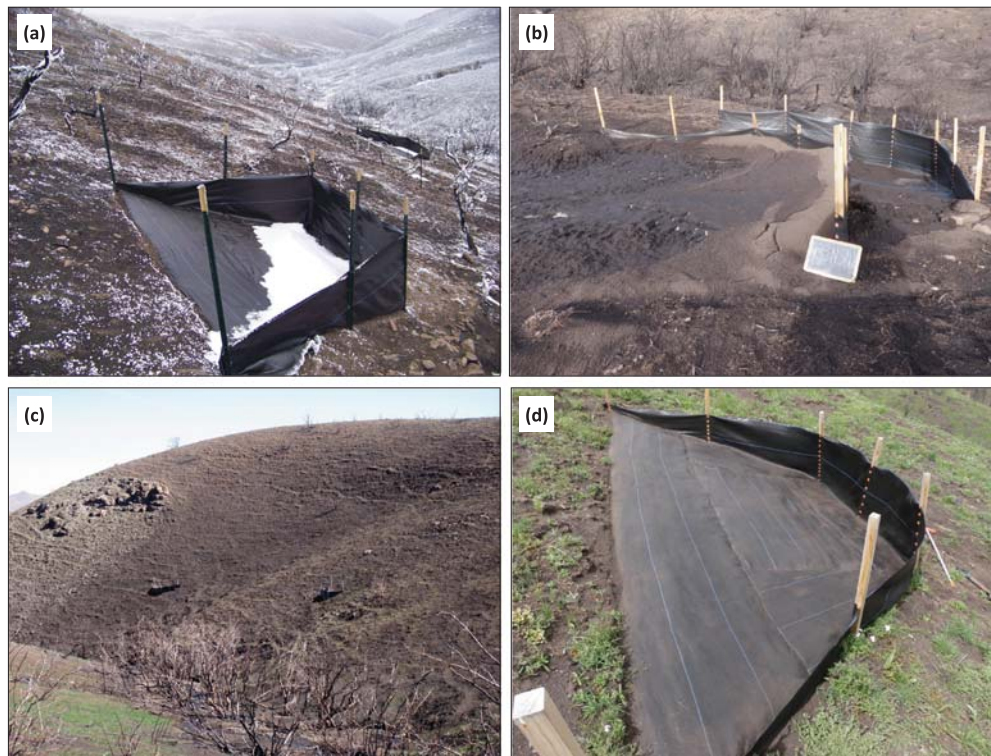
Figure 6. Photographs of silt fence designs in the Murphy Creek Experimental Watershed installed in the months following the 15 August 2015 Soda Fire. Panel (a) shows a short-hillslope plot silt fence on a south aspect with frozen soils in late November 2015; panel (b) shows the dual silt fence design in a swale plot on a north-facing hillslope, with sediment from runoff of rainfall on frozen soils as observed in late November 2015; panel (c) shows a north-facing hillslope with one long-hillslope plot and one short-hillslope plot in early April 2015 (~9 months post fire); and panel (d) shows a long-hillslope plot silt fence on a north-facing aspect in May 2016, approximately 10 months post fire. Photos by US Department of Agriculture, Agricultural Research Service, Northwest Watershed Research Center. [Colour figure can be viewed at wileyonlinelibrary.com ]
