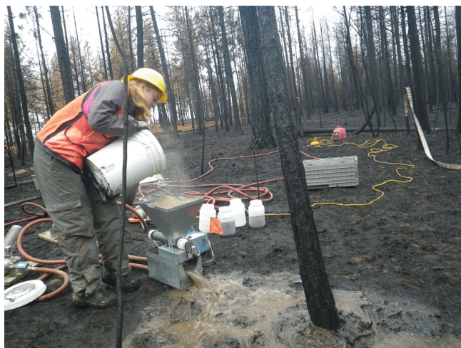
FIGURE 3 Sediment being added to the sediment hopper which was calibrated to add 25 g/L of sediment to the three flow rates
