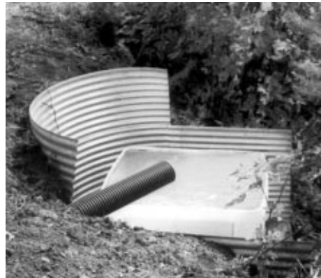
Figure 4. Culvert pipe and collection bucket used to measure soil erosion.
