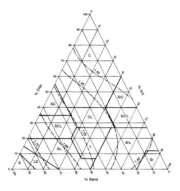
Figure 3.--Growth-limiting bulk density textural triangle.
