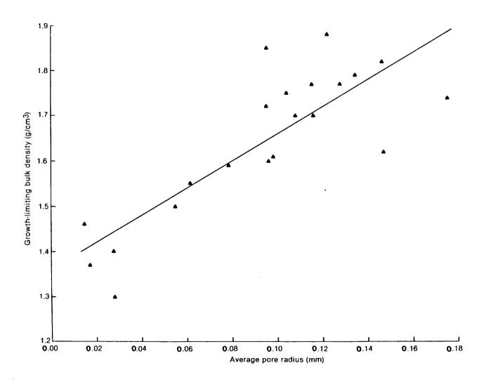
Figure 2.--Relationship between growth-limiting bulk density and calculated average pore radius.
