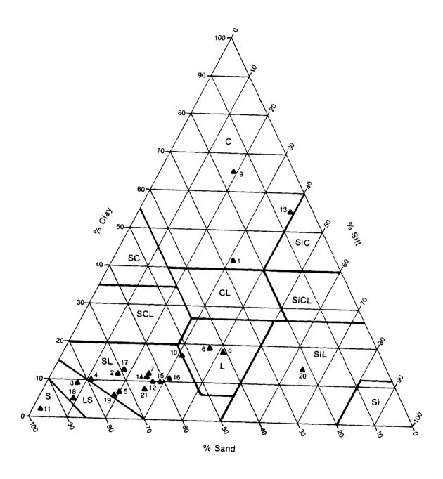
Figure 1.--Distribution of soil textures having growth-limiting bulk density values. Numbers 1-21 inside the triangle refer to soil data numbers in Table 1.
