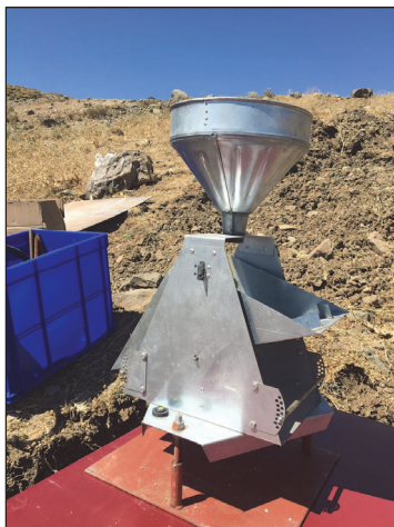
Figure 8. Tipping bucket runoff measuring device like those installed in the pits below the erosion plots (figs. 6 and 7) to measure runoff rates on the Red Mountain Burn Erosion study (photo by A. Yuksel).
