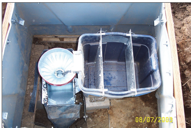
Figure 7. Sediment basin and tipping bucket device installed in enclosure downhill from the bordered erosion plot (figs. 5 and 6) on the Red Mountain Burn Erosion study (photo by I. S. Miller).
