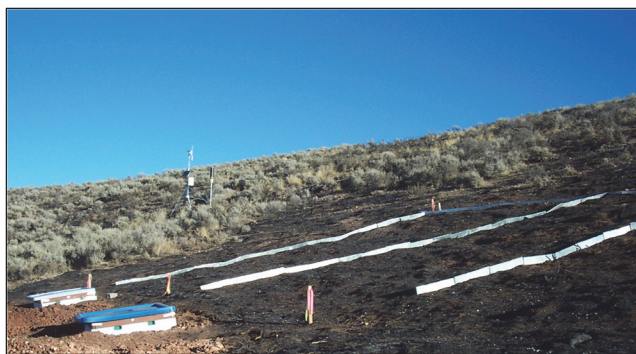
Figure 5. Installation of the plot borders on two of the burned plots on Burn Unit 11 in October 2003. On the lower left are the covers over the boxes containing the sediment basins and tipping bucket devices (fig. 7). The bottom gutters to divert runoff and sediment from the bordered plots to the sediment basins (fig. 6) have not yet been installed. The weather station is in the background still on Burn Unit 11, but the burn was less severe on the Red Mountain Burn Erosion study (photo by I. S. Miller).
