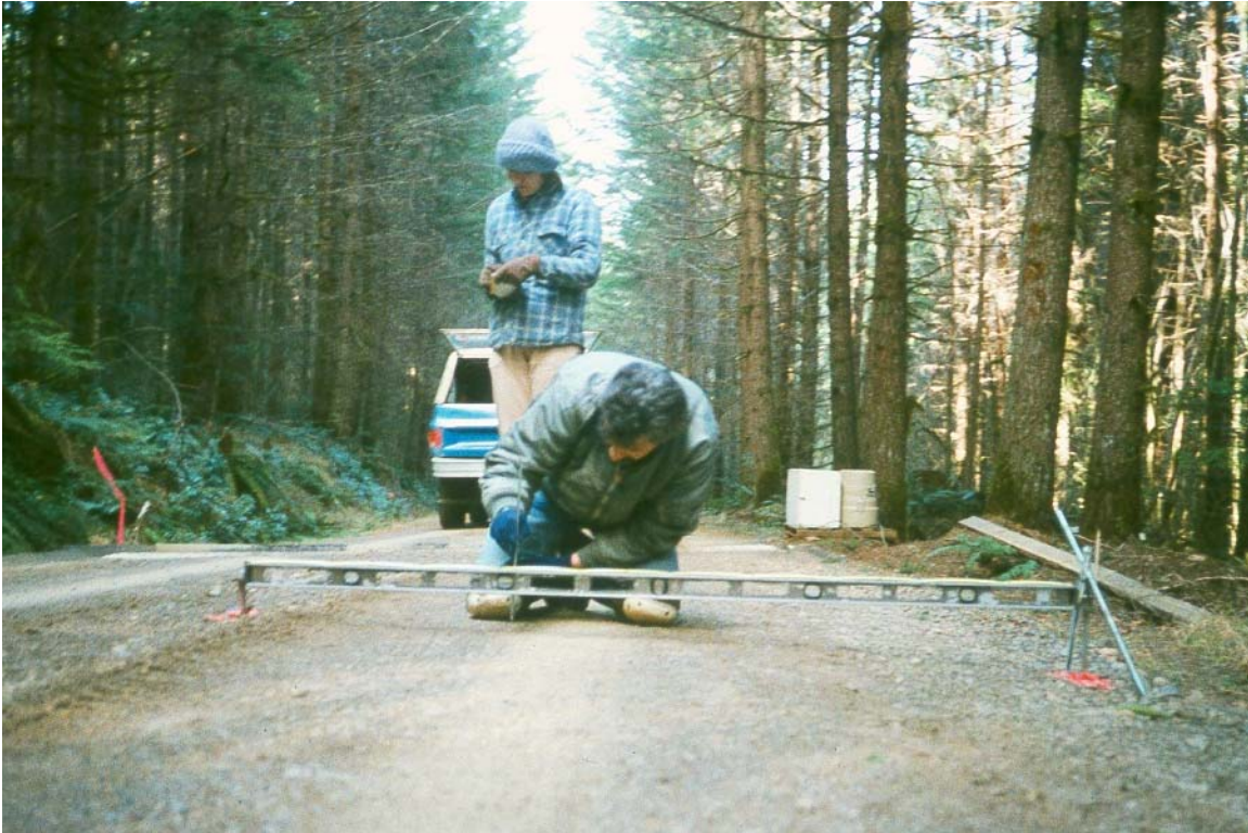
Figure 2. Measuring rutting on a road in the Willamette National Forest, OR.
