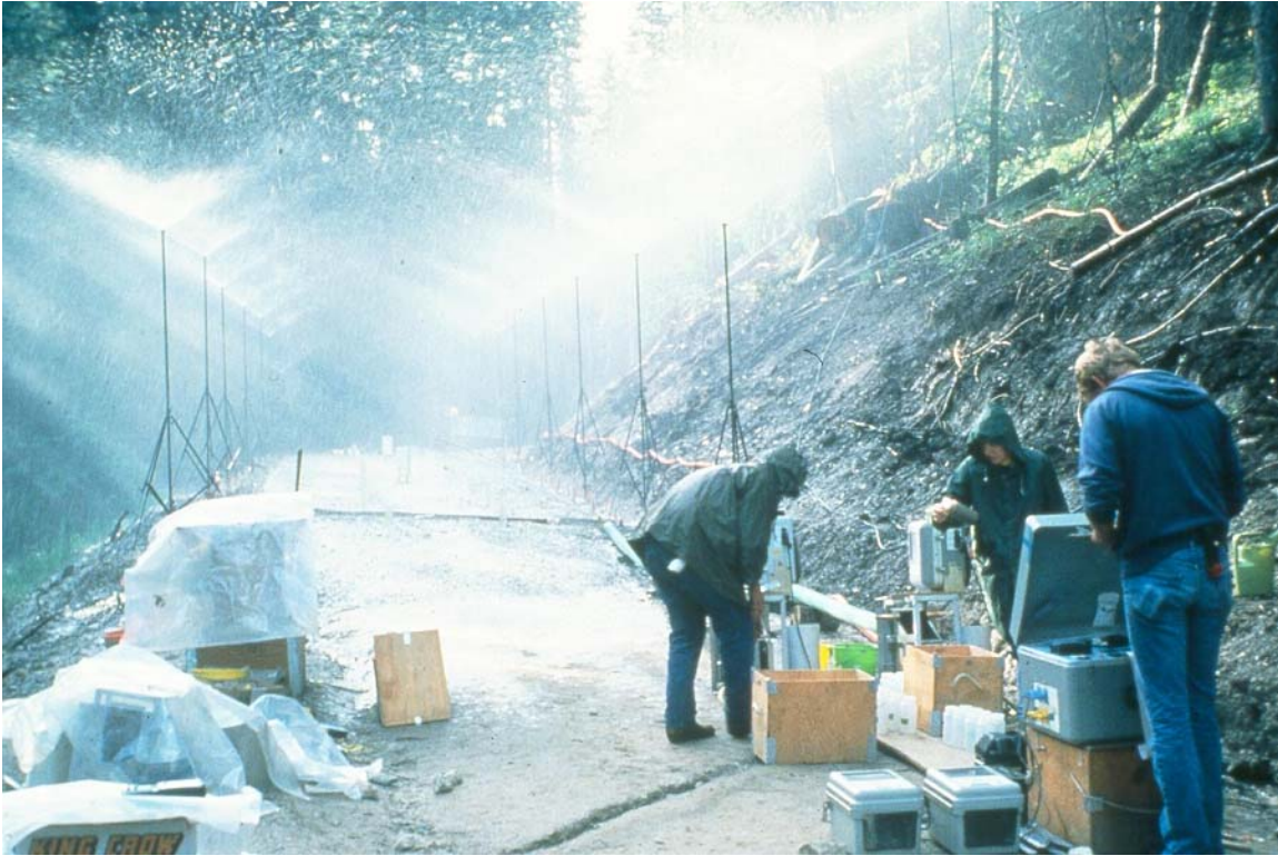
Figure 1. Measuring road erosion rates in central Idaho with a rainfall simulator.
