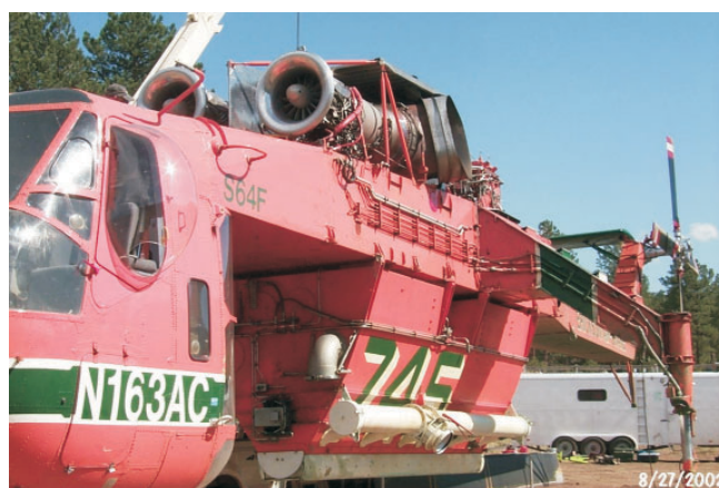
Figure 8 —Helicopter with tanks for hydromulch slurry.
