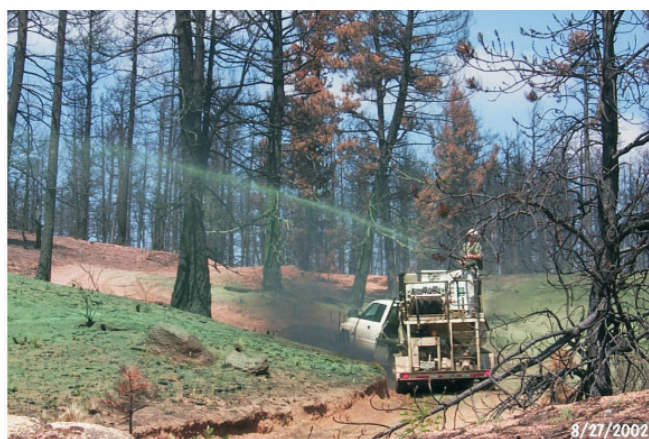
Figure 6 —Ground-based application of hydromulch with seed.
