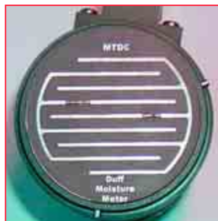
Figure 3—The bottom of the sample chamber is a printed circuitboard containing two interlocking finger sensor electrodes attached to a movable piston.
