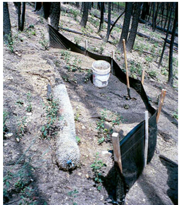
Comparing the effectiveness of a straw wattle after the 2000 Bitterroot Valley fires.
