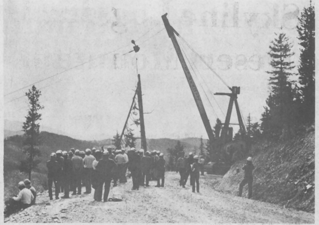
ROYAL LOGGING'S SKAGIT Operator is Tom Albert with hookers, Bob LOGGER was viewed by men. Running cable system reduces terrain damage. Albert, Bud Koppy and Chuck Major.
